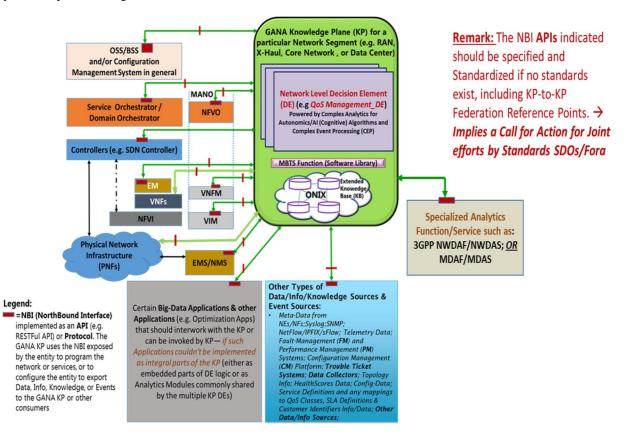
Figure 2: The Integration of the GANA Knowledge Plane (KP) with various management and control systems through which the Knowledge Plane can selectively program the network and KP integration with Event Sources, Data Sources and Info/Knowledge Sources
