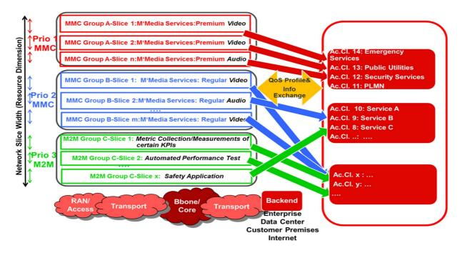
Figure 18: Illustration of the concepts of Network Slice Width; Slice Prioritization; Services Grouping and allocation to Slices; and Access Class List (Ac.CL) mappings to Flow-Oriented (Flow-Level) Services (e.g. Customer IP Flow Services and Telemetry Services, Performance Test Services and specialized Application Flows) running within a particular Slice
