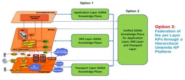
**NOTE:** Types of GANA DEs that should be instantiated in specific KP depends on the Types of Managed Entities in associated Layer
