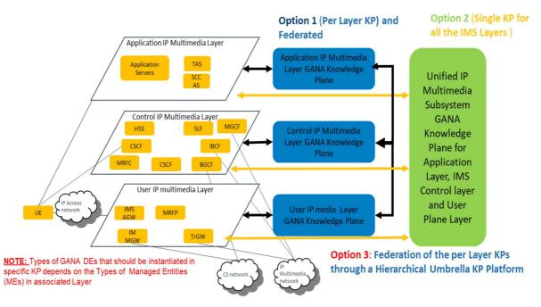
Figure 10: Options that may be pursued in implementing GANA KP Platform(s) in IMS environment architecture Scenario-1
