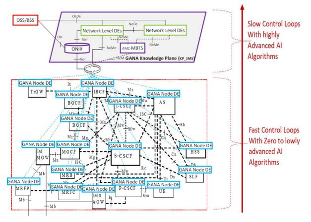
Figure 9: Block diagram of GANA instantiation onto the IMS architecture, GANA Decision Elements (DEs) in Autonomicity-enabled IMS Architecture
