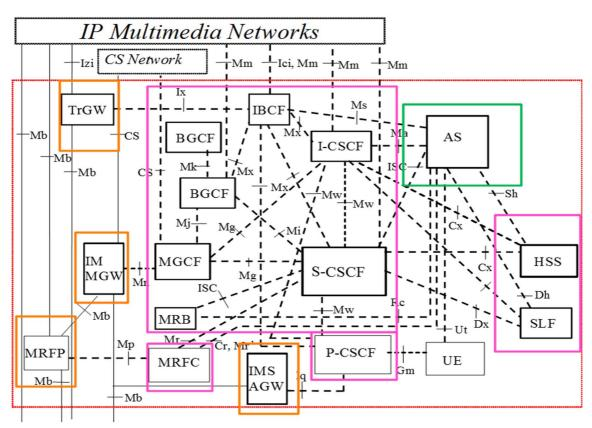
Figure 6: ETSI TS 123 228 [i.1] Reference Architecture of the IP Multimedia Core Network Subsystem
